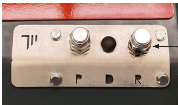
Image 5. Hydraulic ports for connecting the hydraulic hoses.
