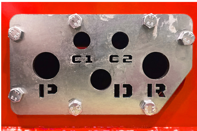
Image 4. Image of the bushings for connecting the mulcher head's hydraulic hoses.
