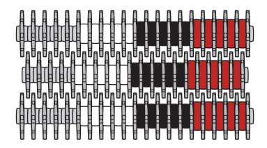
Achieve precise screening capabilities thanks to the use of spacer rings. Quickly modify your bucket without disassembling the shafts.
