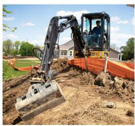
Whether you are digging pools, ponds, sidewalks, foundations, hardscapes, utility trenches, swales, or drainage ditches the Mongo Attachments Hydraulic Tilt Bucket will get the job done faster and more precisely. Mongo tilt buckets come ready to use, with the appropriate length hoses and flat-face couplers included.
