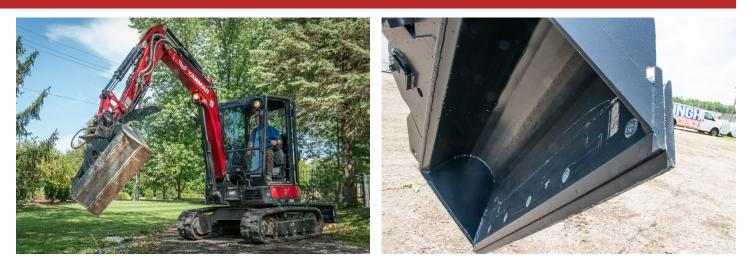
Whether you are digging pools, ponds, sidewalks, foundations, hardscapes, utility trenches, or anything else, take your mini excavator to the next level with the Mongo Attachments Hydraulic Power Tilt Bucket. Our fine leveling feature allows you to dig level grade from uneven surfaces. With 45 degrees of tilt in both directions, this bucket gives you the versatility to dig hard to reach areas and extreme angles.
